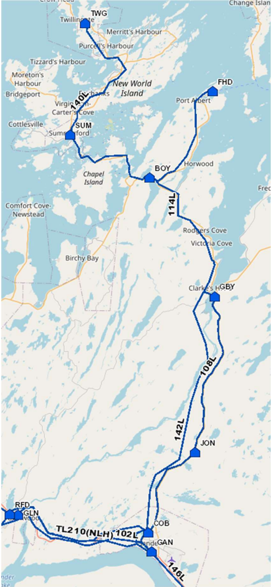
Figure B-2: Gander Bay 66 kV Transmission System
